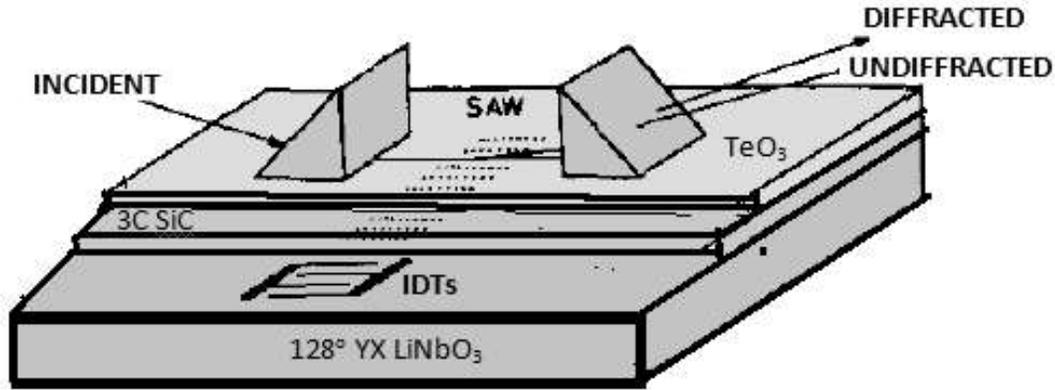
**Figure 1: TeO<sub>3</sub>( )/3C-SiC()/128°Y-X LiNbO<sub>3</sub> multilayered acousto optic device configuration with IDTs placed on the top of LiNbO<sub>3</sub> crystal.**
