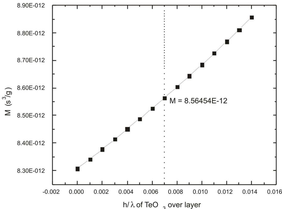
**Figure 3: Variation of figure of merit with TeO<sub>3</sub> over layer thickness in TeO<sub>3</sub>/3C-SiC()/128°Y-X LiNbO<sub>3</sub> SAW layered structure.**
